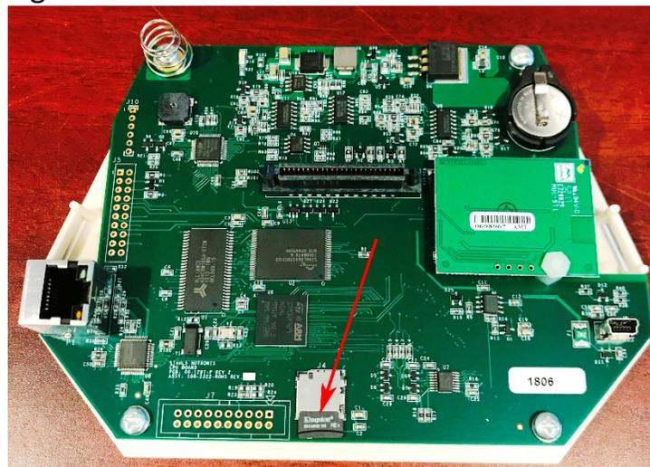
6) Remove the existing SD card and install the new one.
