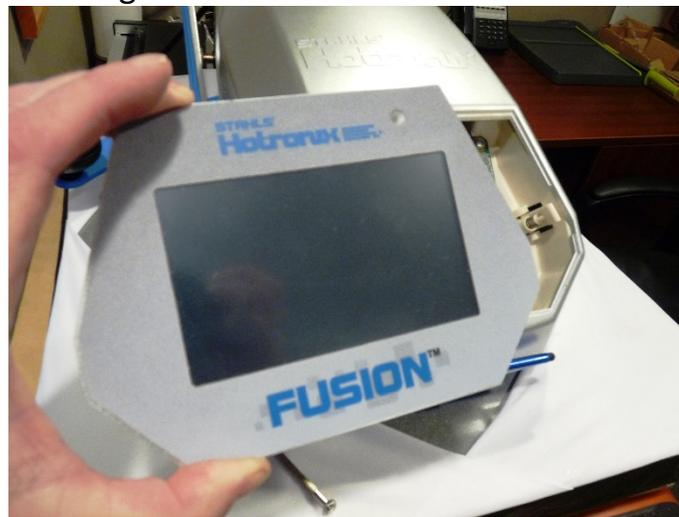
5) Turn the display enclosure over. There will be a MicroSD card on the bottom-center of the unit's motherboard. See Figure 6
