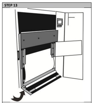
Place the paper three quarters of the way up the path so the paper has covered the paper sensors completely.
