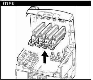
Remove the four image drums/toner cartridge units and place them on a flat surface.
