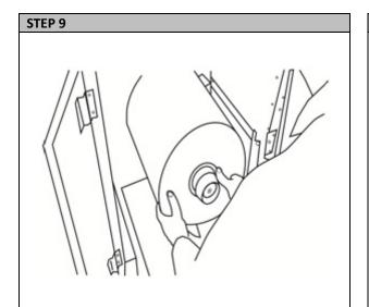
Open the Media Door. Insert a roll of 12.90" (327.66mm) paper as shown, ensuring you're holding the roll on the side and making sure the core is flush with the media. Ensure the outside edge of the roll is flush with the inside core. If this is not done properly, there will be tracking problems. Ensure the roll is pushed all the way into the feeder against the back Extension Arm.
