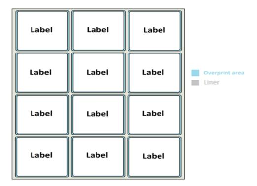
The Trim Box is the size of the die cut label. The die cut dimensions are of course the choice of the printer and can be ordered from any converter.
