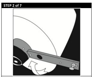
Lift the Extension Arm back up into position making sure both the Plunger and Extension Arm lock.
