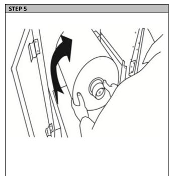
Open the Media Door of the feeder. Lower the Extension Arm. Using both hands, rewind the paper roll until the yellow LED light on the feeder menu begins flashing. At this time, you want to ensure the tension on the paper roll isn't too tight and the roll isn't damaged or coning.
