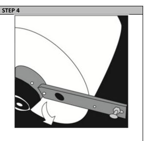
Open the Media Door. Pull the plunger to release the Extension Arm. Drop the Extension Arm down, and remove the media roll if one is loaded:
