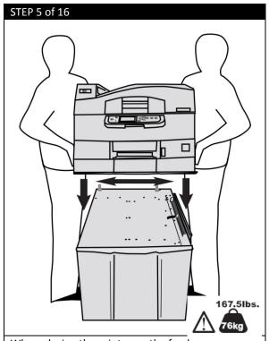
When placing the printer on the feeder, ensure you are aligning the printer with the pins located on the top back of the feeder.
