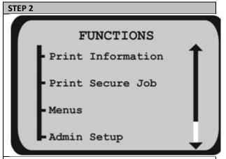
Press **Menu** on the printer display panel to enter the printer menu. Scroll down and select **Admin Setup** to enter.
