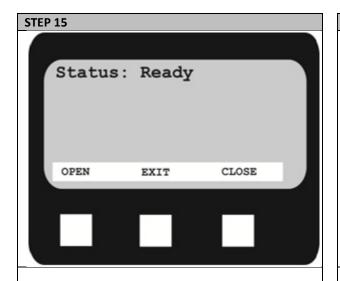
PRESS and HOLD the **Exit** button for 3 seconds to exit out of the guide adjust mode.
