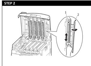
Use the LED cleaner provided with the toner cartridges or a soft, lint-free cloth to gently wipe each of the four heads (1). Move the cleaner as shown, using a fresh section for each pass. Be careful not to damage the guards (2). When finished, close the top cover.
