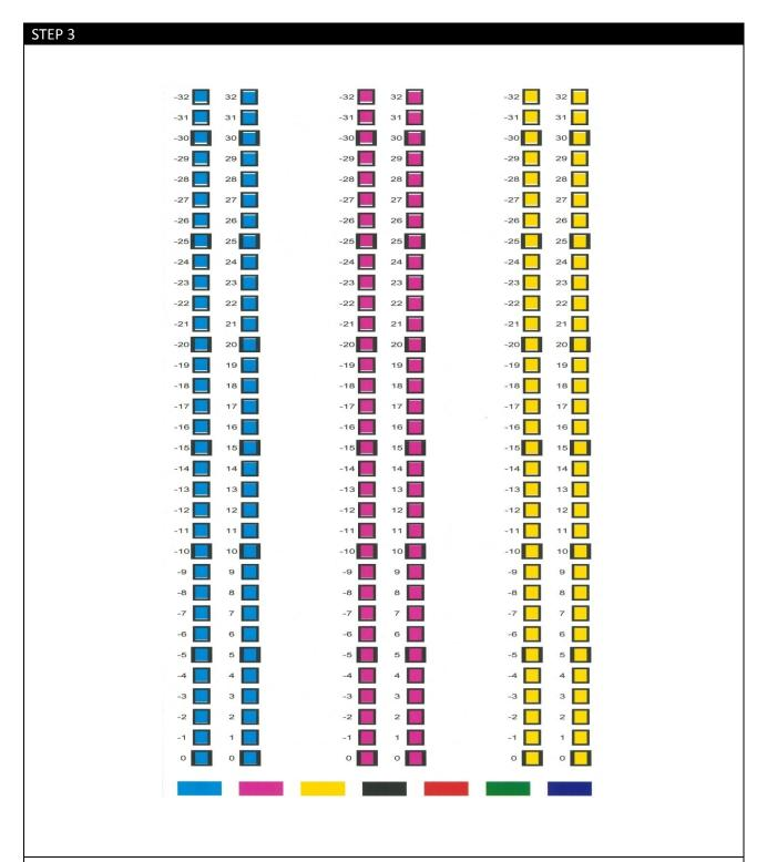
The printer will print a similar page that will aid in determining the proper registration values across CMY. Using a printer's loupe, or best judgment, the correct values can be determined. In this case, the correct values are as follows: C:6 M:4 Y:0; this is because the pixels are perfectly filled within the boxes.
