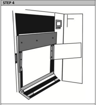
Open the Guide Door and Guide Cover. Open the two Guide Channels and Load Door.
