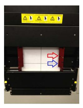
**Red Arrow**: Where the sensor is located. The media needs to pass through here to be calibrated.
