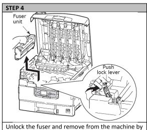
Unlock the fuser and remove from the machine by lifting upwards.
