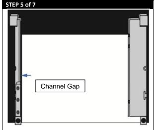
Ensure the Channel Gap (the distance between the edge of the paper and the Guide Channel) is less than 0.5mm on each side and the paper aligned with the right side Guide Channel.
