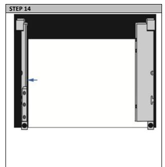
Ensure the Channel Gap (the distance between the edge of the paper and the Guide Channel) is less than 0.5mm on each side and the paper aligned with the right side Guide Channel.
