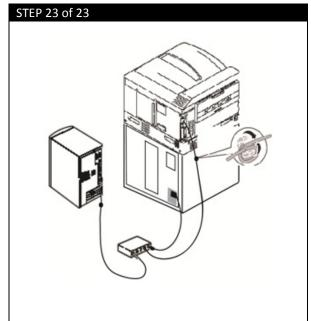
In order to reduce electromagnetic interference—"noise" that interferes with TVs or other appliances—you must place the included ferrite core on the network cable.
