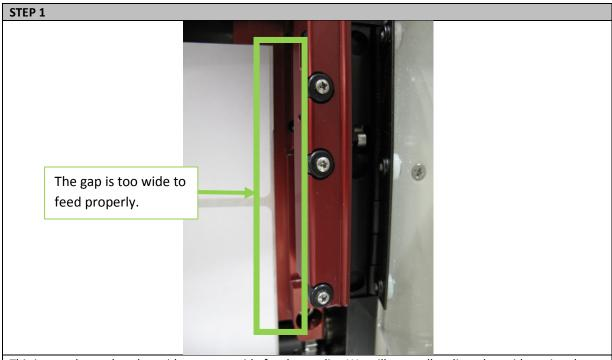
This image shows that the guides are too wide for the media. We will manually adjust the guides using the panel on the feeder.
