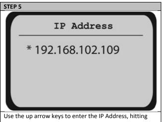
Use the up arrow keys to enter the IP Address, hitting enter to move right to the next column. When a \* (asterisk) symbol appears, the IP Address has been saved. Select **Online** to finish.
