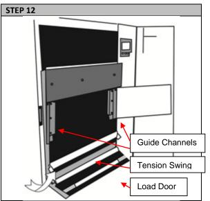
Open the Load Door at the bottom front of the feeder by releasing the two yellow latches.
