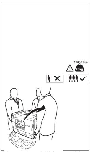
Using two or three people, lift the printer and place it on the feeder, making sure the printer is level on the feeder.
