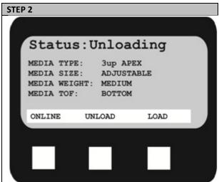
Press the **Online/Offline** button which will cause the feeder to unload the media (it will do this if there is media loaded or not).
