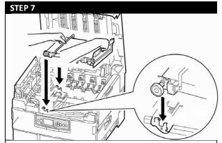
Unpack the new transfer belt, grasp the blue handles and lower the left side of the belt into the printer, fitting the pins into the guides at the front and back, then lower the right side.
