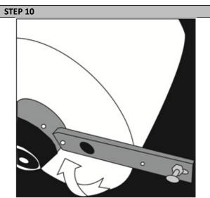
Lift the Extension Arm back up into position making sure both the Plunger and Extension Arm lock.
