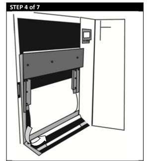
Place the media three quarters of the way up the path so it has covered the paper sensors completely.
