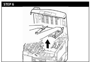
Grasp the blue handles and lift the transfer belt out. Dispose of it in accordance with local regulations.
