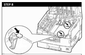
Push down on the belt latches to lock the new belt in place.
