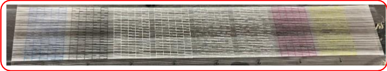
Nozzle check pattern printed in normal nozzle condition.
